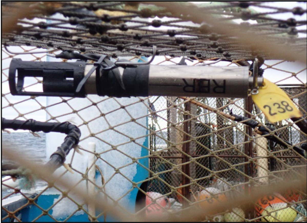
Figure 6. -- An RBR Ltd. XR-420 CTD datalogger affixed to the roof of a crab-survey pot used to capture red king crab ( Paralithodes camtschaticus ) during the 2023 Bristol Bay (Alaska) Collaborative Pot Sampling (CPS1) survey ( photo credit: Vicki Vanek, ADF&G). CTD = Conductivity (i.e., an indicator of salinity), Temperature, and Depth meter.
