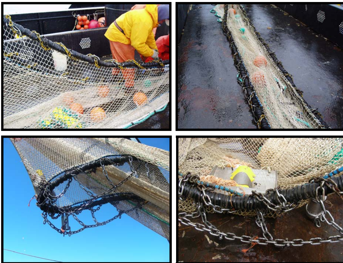
Figure 8. Photos from the 2007 BSFRF trawl showing footrope configuration along wing sections (upper) and the throat section (lower).
