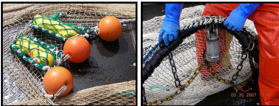
Figure 9. NETMIND sensors (left) and improved modified bottom contact sensor (MBCS) (right) as used in the BSFRF 2007 survey.
